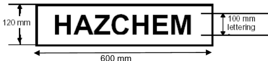
Figure 13.1 Form and dimensions of outer warning placard
